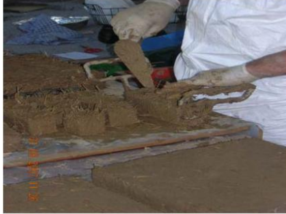
Figure 5 Production of straw bale reinforcement
